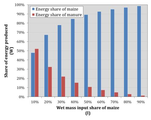
Figure 2 presents the relationship between  $I_n\, \text{and}\,\, W_n$  for the example in which manure and maize are co-digested.
