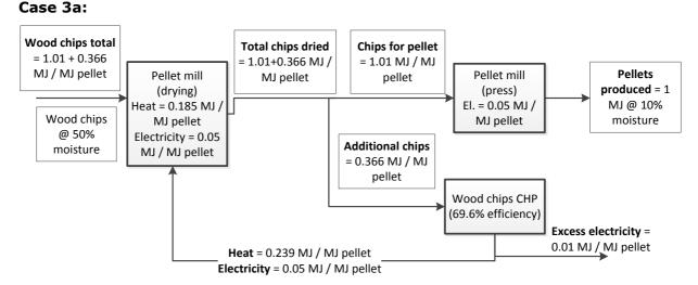
In the case of a CHP engine fuelled with wood chips it is not possible anymore to dimension the CHP on the power needs only, because the heat requirement would not be fulfilled. Therefore, the CHP is dimensioned over the heat demand and an excess electricity is exported to the grid.
