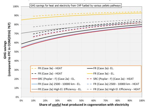
**Figure 16.** Default GHG emissions for electricity and heat co-generated from a Rankine cycle fuelled by pellets as a function of the share of available heat which is exported as useful heat at different temperatures. The pellet production pathways consider a transport distance of 500 km by truck. Two alternative configurations are explored: the blue lines represent the same case as
