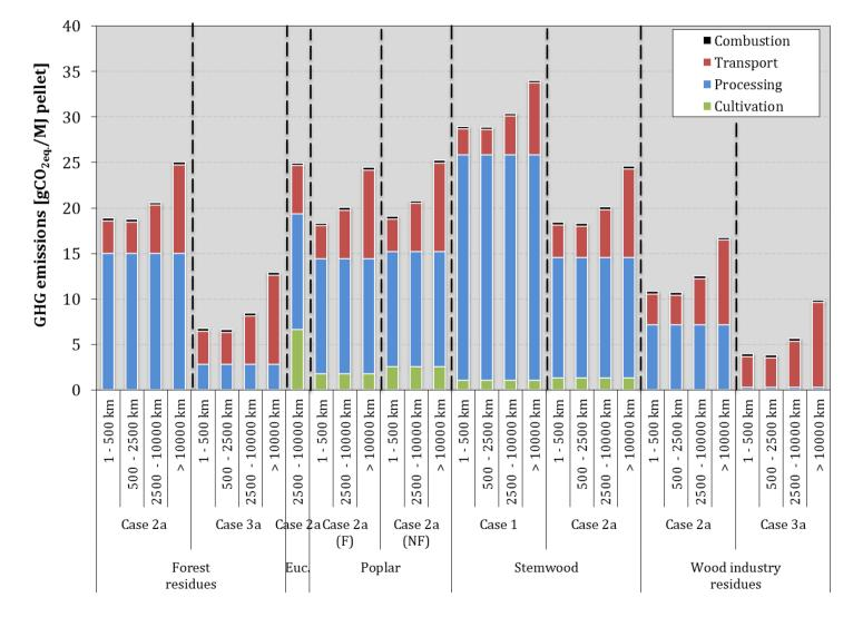
**Figure 4.** GHG emissions for the most relevant wood pellets pathways: contribution of various steps in the supply chain. Based on the default values reported in Table 88, Table 89, Table 92 and Table 93.
