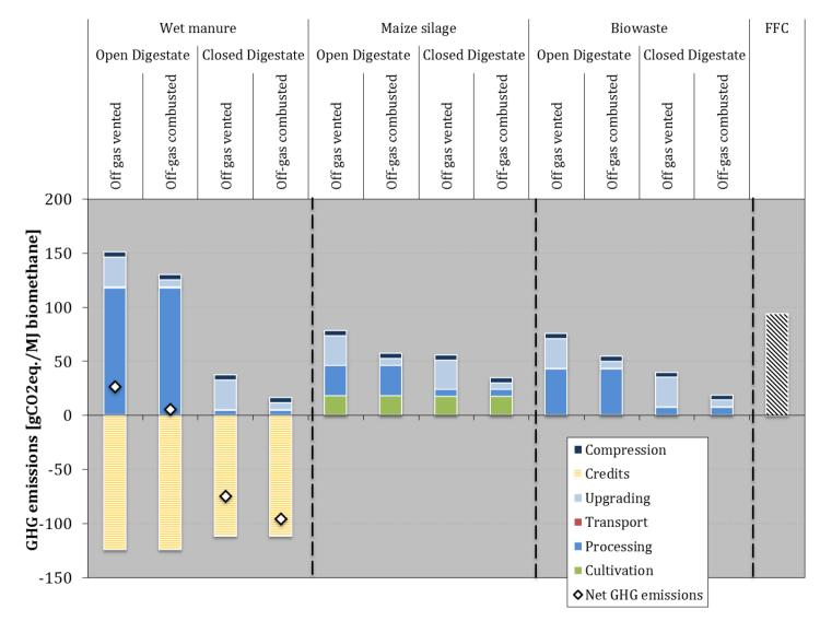
**Figure 8.** Default GHG emissions values for the production of compressed biomethane. FFC considered is equal to 94 gCO<sub>2 eq.</sub>/MJ. Substrate characteristics are the ones detailed in Part Three of this document.
