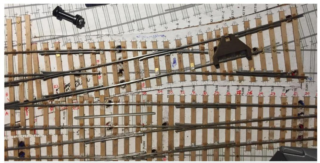
Figure 9 Progressing with the diamond. At least two flangeway gauges are desirable for getting the obtuse crossings right! Both roads are curved, so the common crossings are quite different – 1:8 at one end, and 1:3.4 at the other. The 1:8 is a C&L complete crossing, one of several purchased for such purposes. The big holes for the droppers weren't planned, it's just that I needed a drill bit long enough to clear two layers of ply, cork and pink foam, and the shortest available was 6mm diameter.
