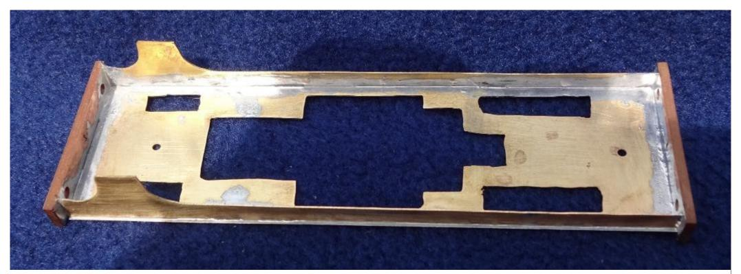
The footplate was fretted out (not very well) and the buffer beams were made up from PCB to give something like the right thickness. The rather curious deep valences were then added.
