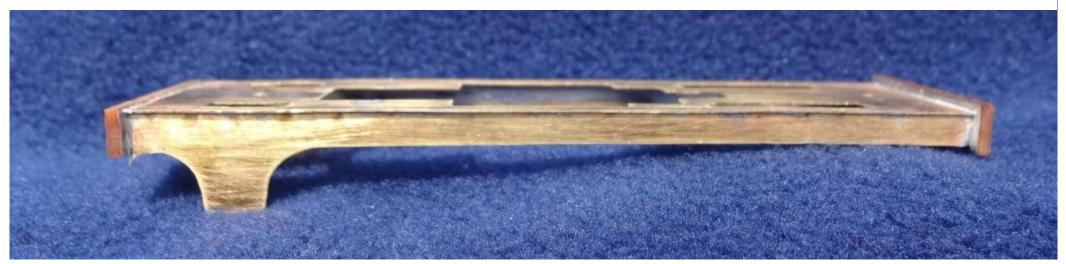
The combined footplate and chassis. It became evident that the rear drive shaft will have to come off. At this point I began to wonder whether a HighLevel gearbox might not have allowed rather more flexibility, rather than the Branchlines box that is shown here.
