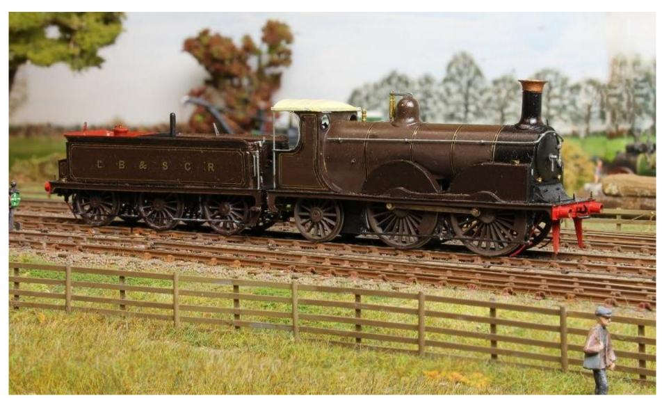
I2 Scratchbuilt using a Mashima motor, High Level gearbox, Sharman bogie and pony wheels and Gibson drivers. It is fully compensated with split axle pick up, Perspex radial axle box and simple bogie pivot. The painting process has been the same as for the E4x but the panels were lined directly using precision lining gold. The upper panels had to be redone using transfers. Painting involved a coat of gloss
