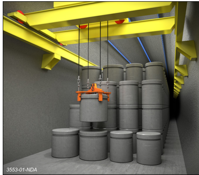
Figure 33 1 cubic metre concrete drums and 500 litre drums stacked in a dedicated vault in a lower strength sedimentary rock
