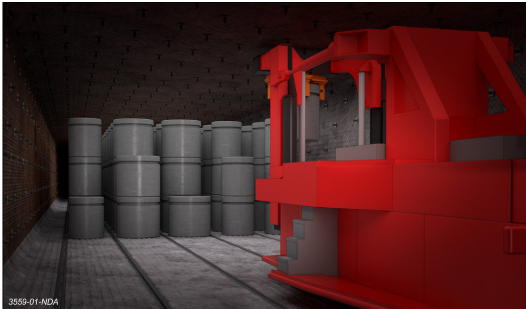
Figure 34 1 cubic metre concrete drums and 500 litre drums stacked in an illustrative dedicated vault in an evaporite rock
