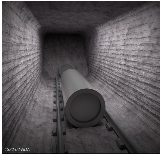
Figure 41 Schematic of a HHGW disposal tunnel – evaporite rock
