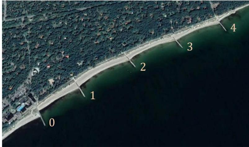
Figure 6.6. Groynes built in Ystad Sandskog west to trap sediment. Orthophoto from 2019. ©GoogleEarth
