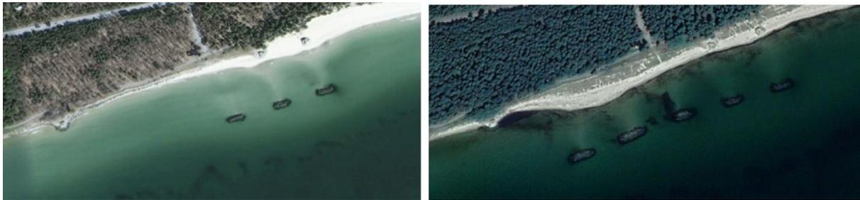
Figure 6.7. Detached breakwaters in Sandskogen east with sediment build-up on the beach side and to the west. Left: The first three breakwaters. Photo from 2010. Right: Two more breakwaters have been built. Orthophoto from 2019. ©Google earth.
