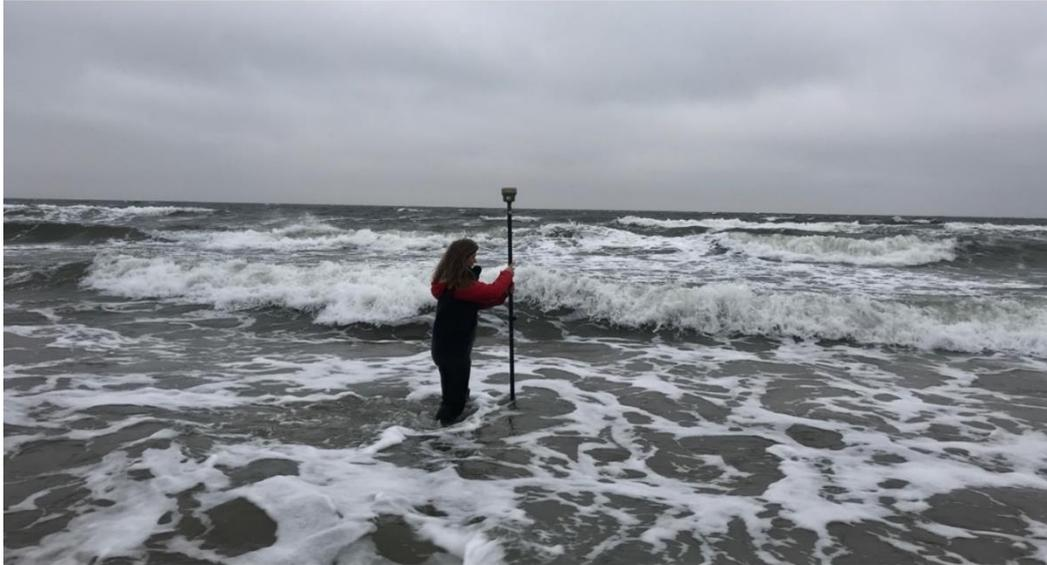
*Figure 5.2. Measuring the beach profile seawards using the RTK-GPS. Photo: Johanna Löwdin, 2020-11-18.*
