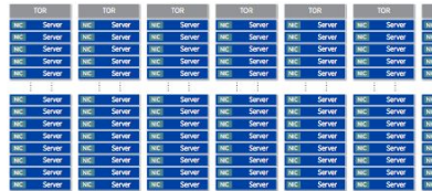
Racks needed to support 2200 VNFs
