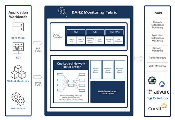
Figure 5: DANZ Monitoring Fabric - Logical Software-Defined NPB
